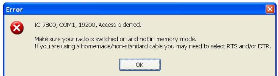
Check that you have not started another radio control program. Other culprits are PDA and mobile phone connections. Even if you have disconnected a device from a COM port you must make sure that the software is no longer running.
